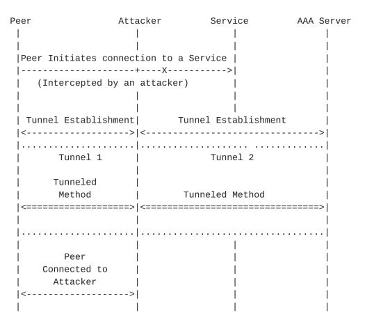
A tunnel t1 extends from the peer to the attacker. a tunnel t2 extends from the attacker to the home EAP server. An inner EAP authentication is forwarded unmodified by the attacker from t1 to t2. The attacker can observe this inner authentication.
