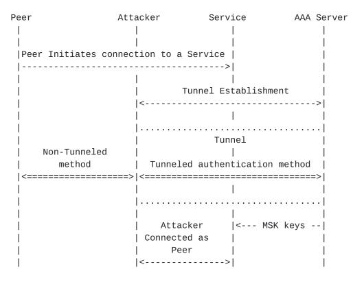
A classic tunnel attack where the attacker inserts an extra tunnel between the attacker and EAP server.
