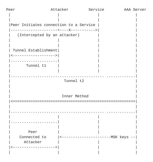
A tunnel t1 from the peer to the attacker contains a tunnel t2 from the peer to the home EAP server. Inside t2 is an inner authentication.
