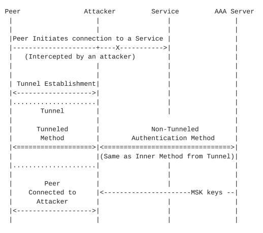
A modified tunnel attack in which an extra server rather than extra client is inserted.
