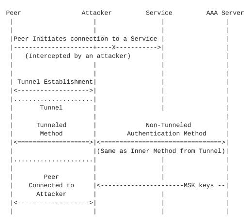
A modified tunnel attack when an extra server rather than extra client is inserted.
