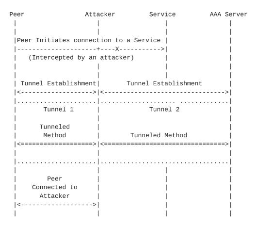
A tunnel t1 extends from the peer to the attacker. a tunnel t2 extends from the attacker to the home EAP server. An inner EAP authentication is forwarded unmodified by the attacker from t1 to t2. The attacker can observe this inner authentication.
