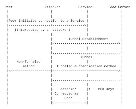
A classic tunnel attack where the attacker inserts an extra tunnel between the attacker and EAP server.
