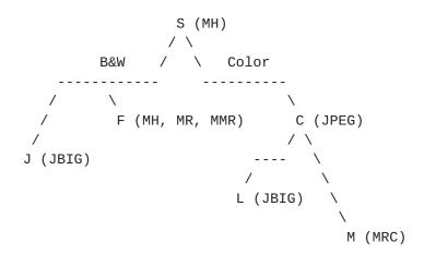
A profile is based on a collection of ITU-T facsimile coding methods. For example, Profile S, the minimal profile, is based on Modified Huffman (MH) compression, which is defined in ITU-T Rec. T.4. Profile F specifies Modified Huffman (MH), Modified Read (MR) and Modified Modified Read (MMR) compressions, which are defined in ITU-T Rec. T.4 and T.6.
