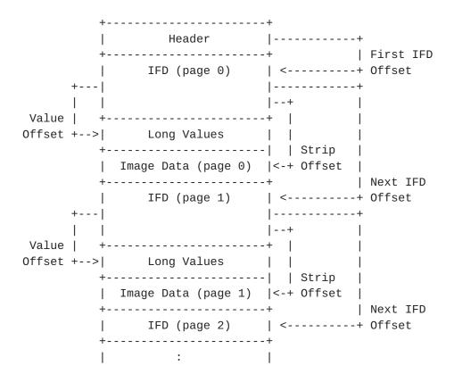
Using this file structure may reduce the memory requirements in implementations. It is also provides some support for streaming, in which a file can be processed as it is received and before the entire file is received.
