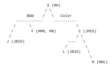
A profile is based on a collection of ITU-T facsimile coding methods. For example, Profile S, the minimal mode, is based on Modified Huffman (MH) compression, which are defined in ITU-T Rec. T.4. Profile F specifies Modified Read (MR) and Modified Modified Read (MMR) compressions, which are defined in ITU-T Rec. T.4 and T.6.
