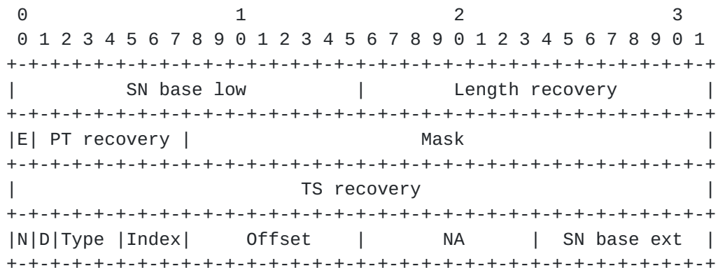
Figure 7: Format of the FEC header
