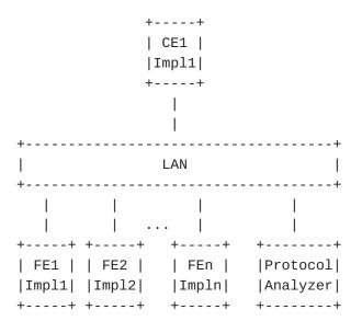
All scenarios were tested more than once with permutation of the CE from different implementors. In the next permutation, the setup were as shown in the following figure.
