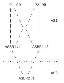
When the session between ASBR1.1 and ASBR2.1 undergoes maintenance, it is required that all BGP routers of AS1 reroute traffic to ASBR1.2 before the session between ASBR1.1 and ASBR2.1 is shut down.
