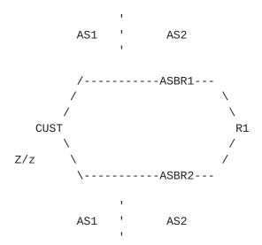
Before the maintenance, packets for destination Z/z use the CUST-ASBR1 link because R1 selects ASBR1's route based on the IGP cost.
