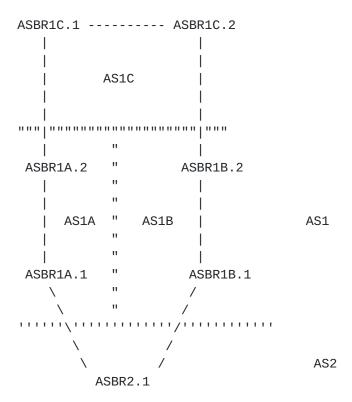
In the above figure, member-AS AS1A, AS1B, AS1C belong to a confederation of ASs in AS1. AS1A and AS1B are connected to AS2.
