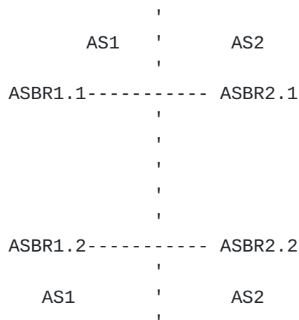
Figure 3. EBGP topology with redundant ASBR in both ASes
