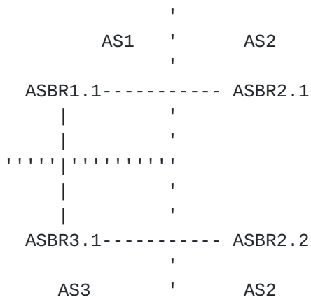
Figure 4. EBGP topology of a dual homed customer
