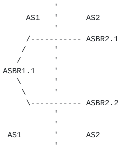
Figure 2. EBGp topology with redundant ASBR in one of the AS.
