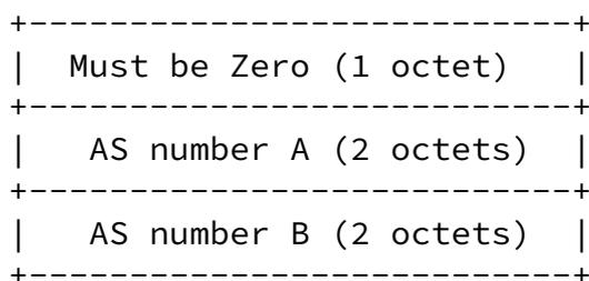
Figure 4: BGP speakers filter containing two distinct two octet AS number
