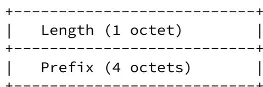
Figure 6: BGP speakers filter containing a CIDR prefix/length pair
