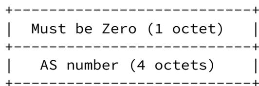
Figure 5: BGP speakers filter containing a single four octets AS number
