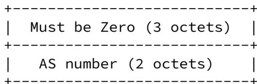
Figure 3: BGP speakers filter containing a single two octet AS number
