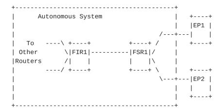
Suppose that FSR1 does not FIB-install routes for which EP1 and EP2 are next hops. In this case, when EP2 sends a packet to FSR1 for which the next hop is EP1, FSR1 will first tunnel the packet to FIR1, which will tunnel it right back to FSR1. This trombone routing is avoided if local ASBRs FIB-install routes where their neighbor remote ASBRs are the BGP NEXT\_HOP.
