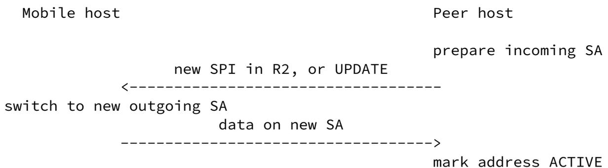
Figure 14: Address activation via use of new SA
