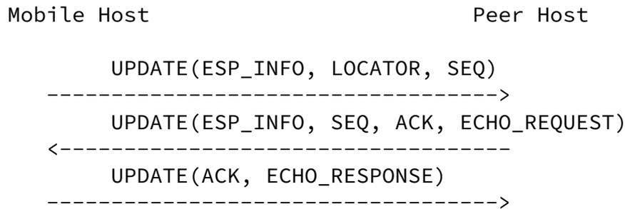
Figure 3: Readdress without rekeying, but with address check
