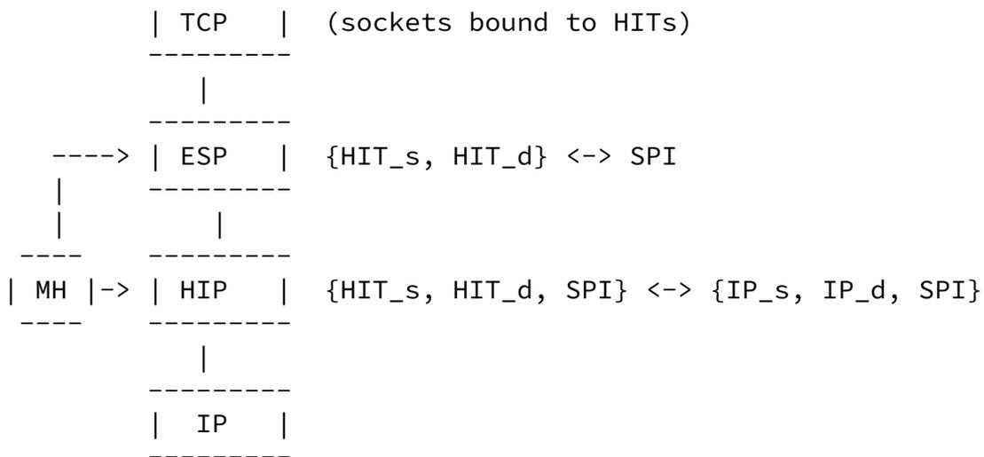
Figure 2: Architecture for HIP mobility and multihoming
