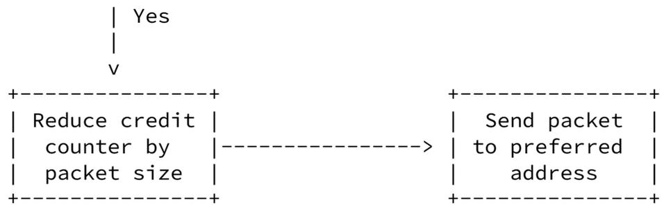
Figure 16: Sending Packets with Credit-Based Authorization
