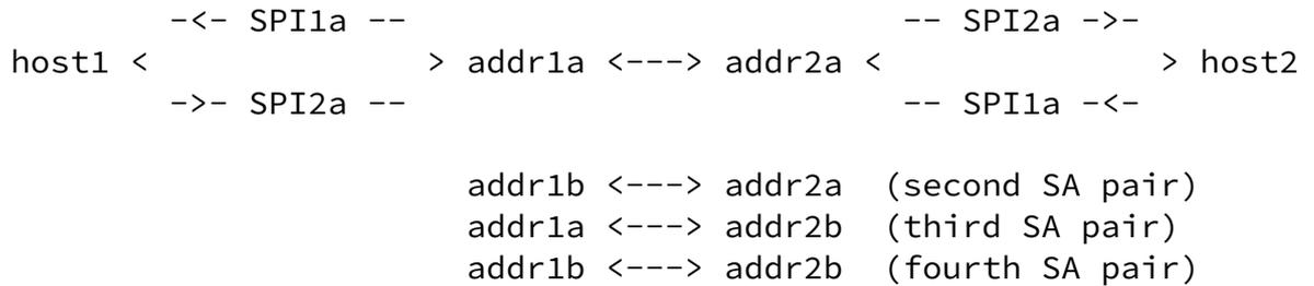
Figure 7: Dual multihoming case in which each host uses LOCATOR to add a second address
