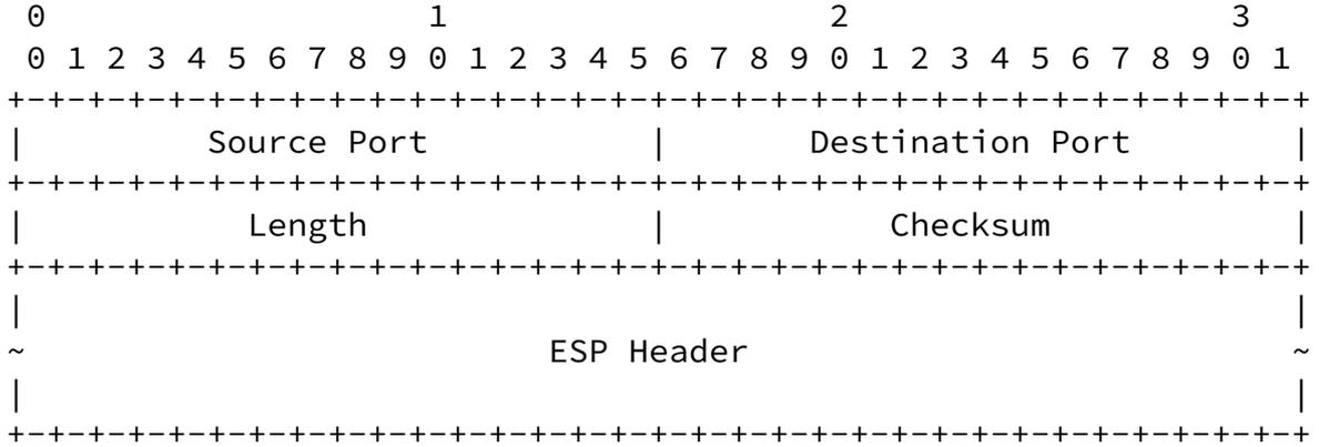
Figure 2: Format for UDP-encapsulated IPsec ESP BEET-mode traffic.
