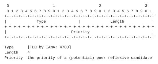
Figure 3: Format of the CANDIDATE\_PRIORITY Parameter
