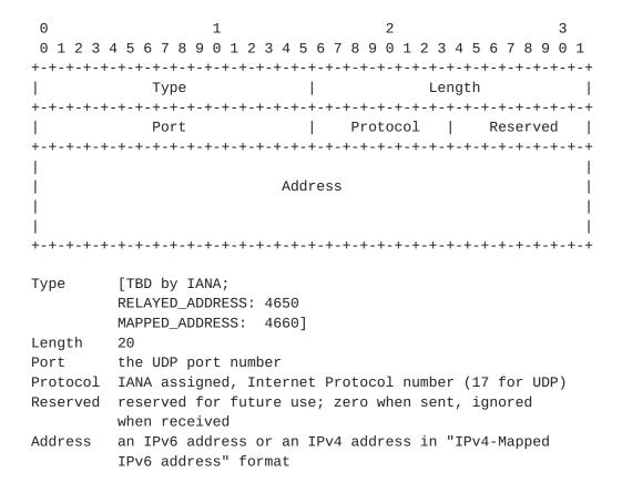
Figure 1: Format of the RELAYED\_ADDRESS and MAPPED\_ADDRESS Parameters
