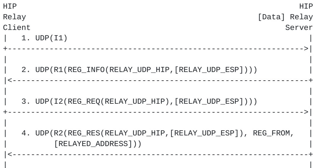
Figure 2: Example Registration with a HIP Relay
