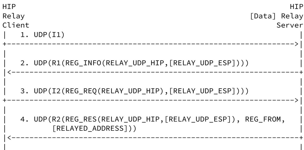
Figure 2: Example Registration with a HIP Relay
