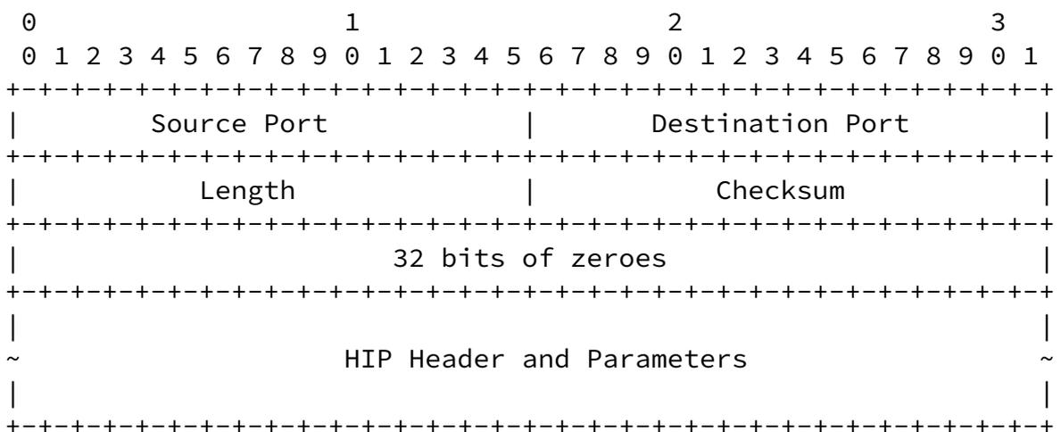
Figure 7: Format of UDP-Encapsulated HIP Control Packets
