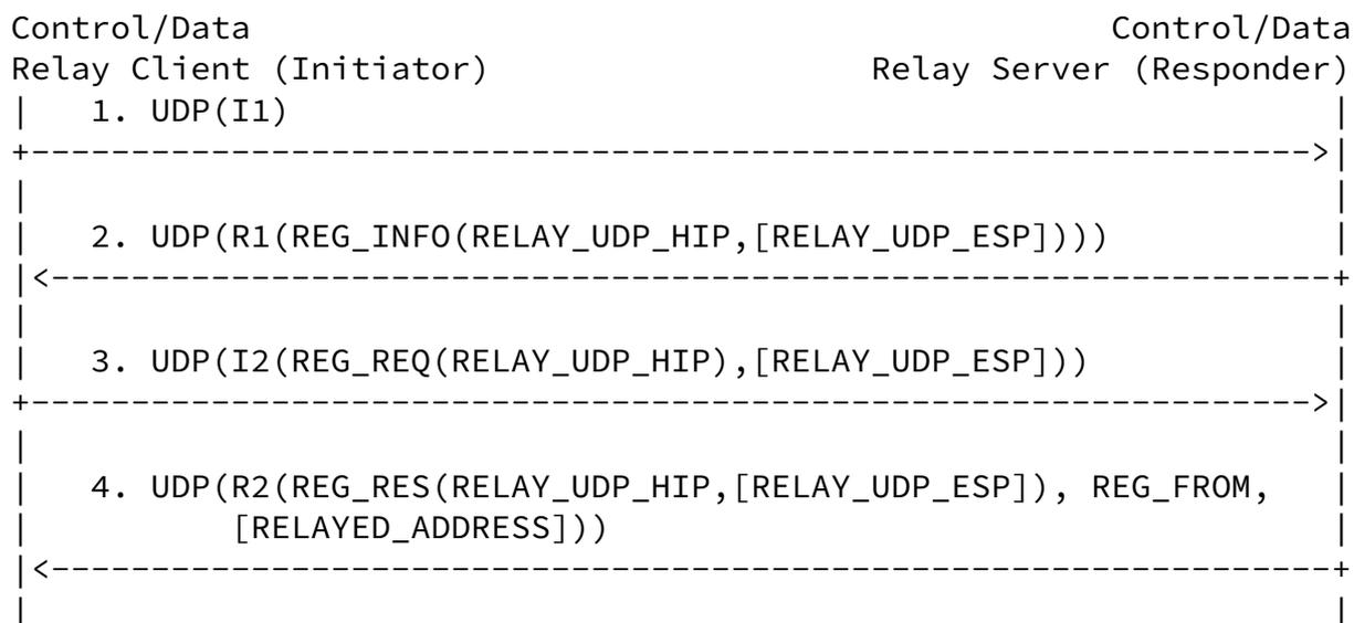
Figure 2: Example Registration with a HIP Relay
