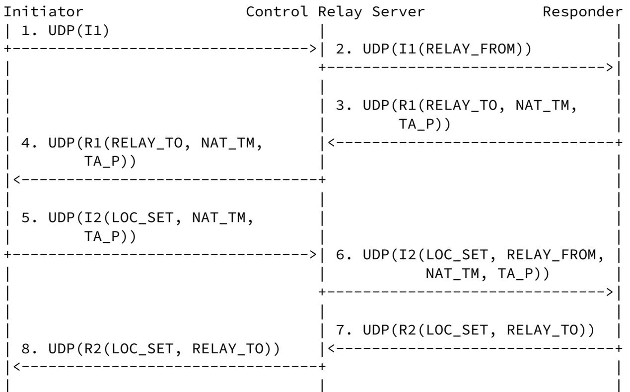
Figure 4: Base Exchange via a HIP Relay Server
