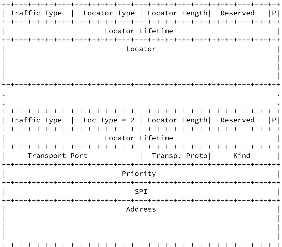
Figure 11: LOCATOR\_SET Parameter
