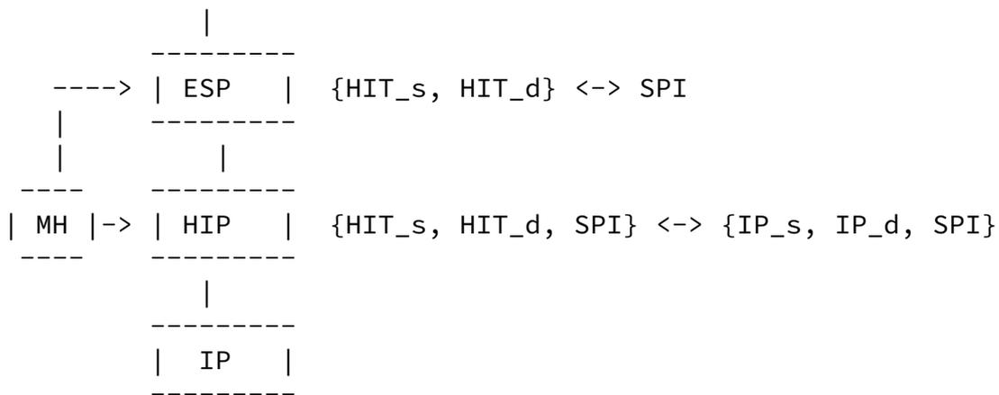
Figure 2: Architecture for HIP Host Mobility (MH)
