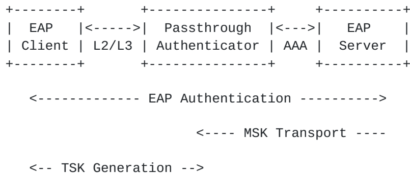
Figure 1: Logical diagram of EAP authentication and key derivation using passthrough authenticator
