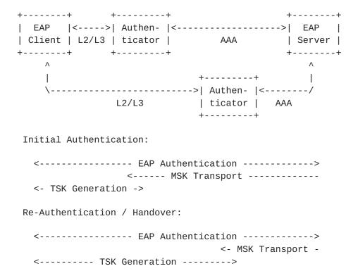
Figure 1: Logical diagram of EAP authentication and key derivation using passthrough authenticator
