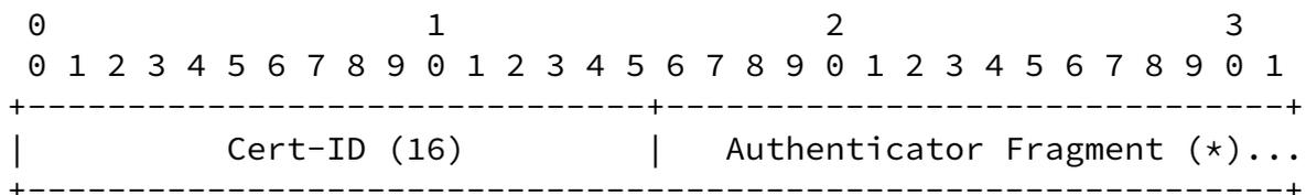
Figure 8: CERTIFICATE frame payload
