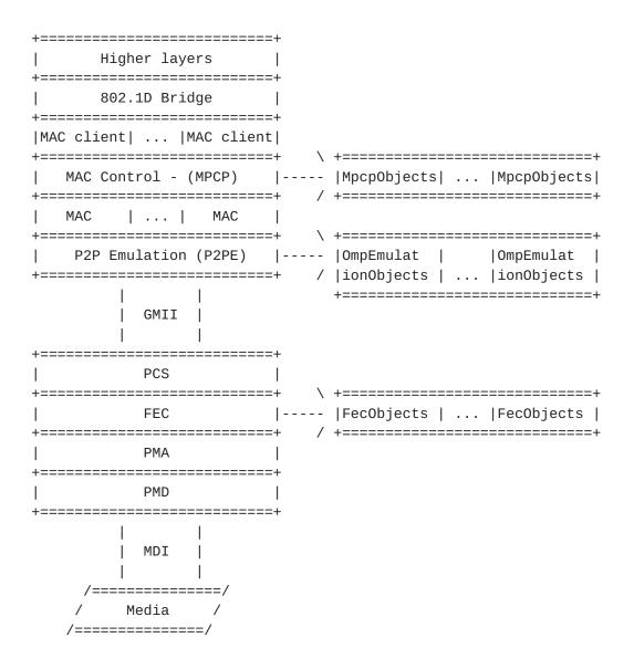
The association is strait forward for the ONU interface. There is one logical and one physical interface and a single copy exists for each layer, that can be remotely queried by the OLT.
