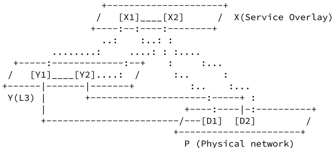
Figure 6: Topology hierarchy example - multiple underlays
