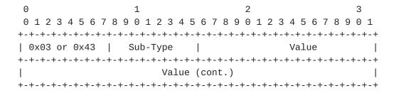
The value of the high-order octet of this extended type is either 0x03 or 0x43. The low-order octet of this extended type is used to indicate sub-types.
