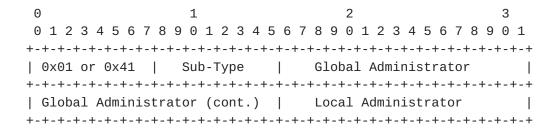
The value of the high-order octet of this extended type is either 0x01 or 0x41. The low-order octet of this extended type is used to indicate sub-types.
