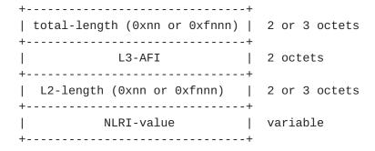
Figure 1: Flow Specification NLRI for L2
