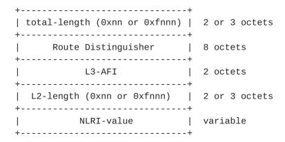
Figure 2: Flow Specification NLRI for L2VPN
