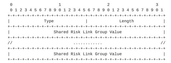
Note that there is no SRLG TLV in OSPF-TE. In IS-IS the SRLG information is carried in two different TLVs: the IPv4 (SRLG) TLV (Type 138) defined in [RFC5307], and the IPv6 SRLG TLV (Type 139) defined in [RFC6119]. In Link-State NLRI both IPv4 and IPv6 SRLG information are carried in a single TLV.
