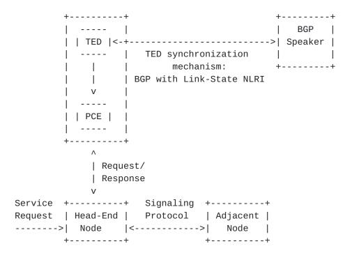
The mechanism in this document allows the necessary TED information to be collected from the IGP within the network, filtered according to configurable policy, and distributed to the PCE as necessary.
