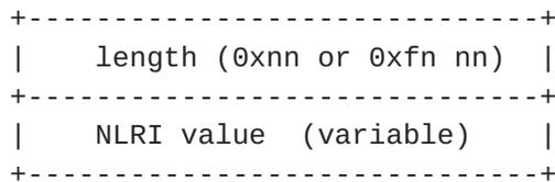
Figure 1: Flow-spec NLRI for IPv4
