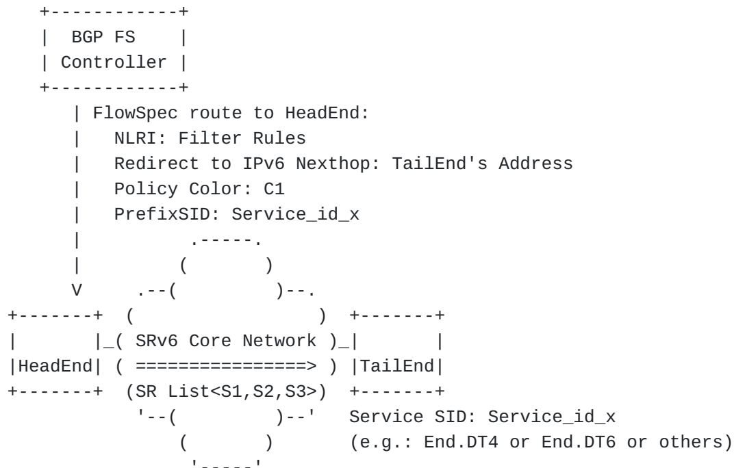
Figure 2: Steering the Traffic Flow into SRv6 Policy (Option 1)
