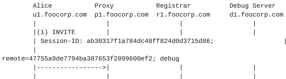
Figure 4: Log-me marking using the "debug" Session-ID: header field parameter
