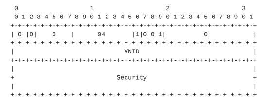
In the above example, the first flag bit is set which indicates that the VNID extension is present; this is a 32 bit field. The second through fourth bits of the flags are paired flags that indicate the presence of a security field with seven possible sizes. In this example 001 indicates a sixty-four bit security field.
