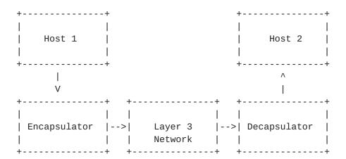
The encapsulator and decapsulator may be co-resident with the corresponding hosts, or may be on separate nodes in the network.
