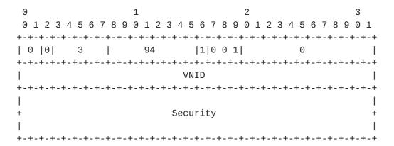
In the above example, the first flag bit is set which indicates that the VNID extension is present this is a 32 bit field. The second through fourth bits of the flags are paired flags that indicate the presence of a security field with eight possible sizes. In this example 001 indicates a sixty-four bit security field.
