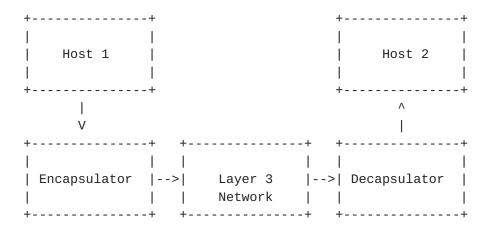
The encapsulator and decapsulator may be co-resident with the corresponding hosts, or may be on separate nodes in the network.
