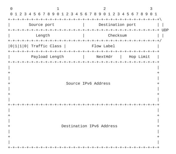
Note that the 0110 value in the first four bits of the the UDP payload expresses the GUE variant as 1 (bits 01) and IP version as 6 (bits 0110).
