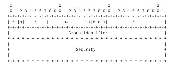
In the above example, the first flag bit is set which indicates that the Group Identifier extension is present which is a 32 bit field. The second through fourth bits of the flags are paired flags that indicate the presence of a Security field with seven possible sizes. In this example 001 indicates a sixty-four bit security field.
