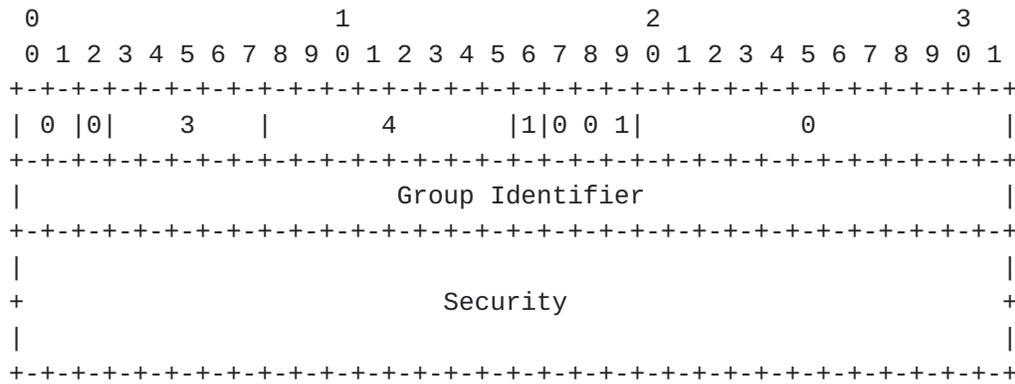
In the above example, the first flag bit is set which indicates that the Group Identifier extension is present which is a 32 bit field. The second through fourth bits of the flags are grouped flags that indicate the presence of a Security field with seven possible sizes. In this example 001 indicates a sixty-four bit security field.
