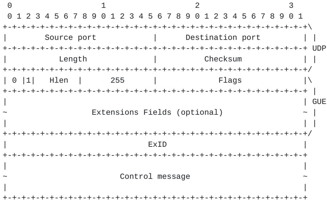
Note that the ExID is not part of the GUE header, it is in the payload. In particular, the ExID is not accounted for in the GUE Hlen.
