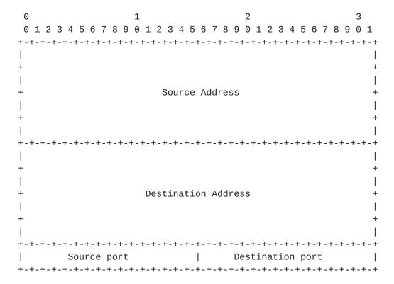
The GUE pseudo header does not include payload length or protocol as in the standard IP pseudo headers. The length field is deemed unnecessary for inclusion because a corrupted length field should not cause mis-delivery, the GUE checksum is applied after GUE fragmentation, and without the length field the GUE pseudo header checksum is the same for all packets of flow.
