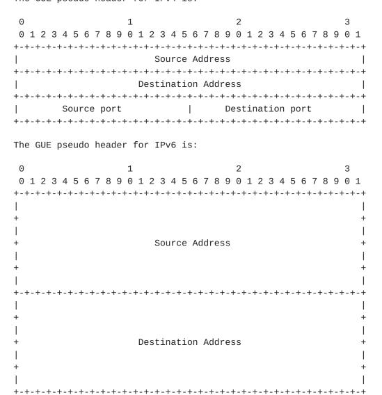
The GUE pseudo header does not include payload length or protocol as in the standard IP pseudo headers. The length field is deemed unnecessary for inclusion because a corrupted length field should not cause mis-delivery, the GUE checksum is applied after GUE fragmentation, and without the length field the GUE pseudo header checksum is the same for all packets of flow.
