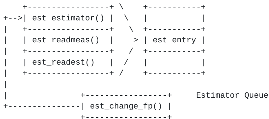
Figure 3: Estimator Unit inside the Kernel
