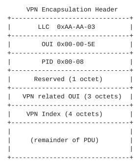
When the encapsulation header is used, the remainder of the PDU MUST be structured according to the appropriate format described in section 5 or 6 (i.e., the VPN encapsulation header is prepended to the PDU within an AAL5 CPCS SDU).
