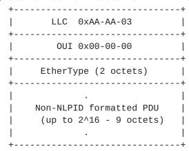
In the particular case of an IPv4 PDU, the Ethertype value is 0x08-00, and the payload format MUST be:
