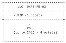
The routed protocol MUST be identified by a one octet NLPID field that is part of Protocol Data. NLPID values are administered by ISO and ITU-T. They are defined in ISO/IEC TR 9577 [6] and some of the currently defined ones are listed in Appendix C.
