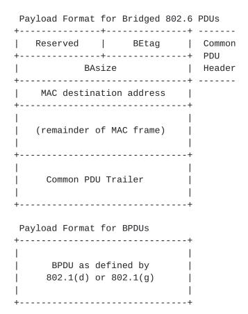
In case of Ethernet, 802.3, 802.4, 802.5, and FDDI PDUs the presense or absence of the trailing LAN FCS shall be identified implicitly by
