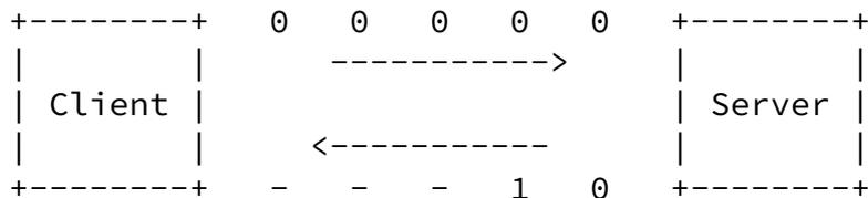
(c) The Server starts sending data and reflects the Delay Sample.
