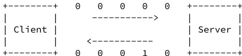
(e) The Server reflects the Delay Sample and so on.
