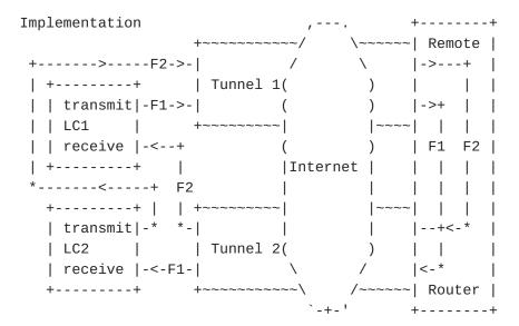
Illustration of a test setup with two layer 2 tunnels. For simplicity, only two linecards of one implementation and two flows F between them are shown.
