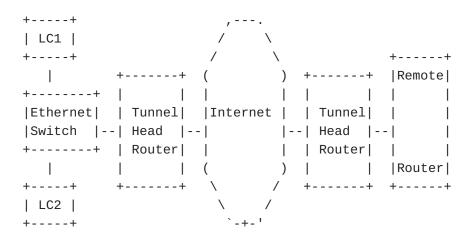
Illustration of a hardware setup to realise the test setup illustrated by figure 1 with layer 2 tunnels or Pseudowires.
