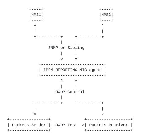
In this architecture, the different NMSÆs query the IPPM-REPORTING-MIB agent for measurements. The agent controls whether the NMS is granted access to perform the measure requested. Each NMS accesses the results of its measurements in the IPPM-REPORTING-MIB statistics table.
