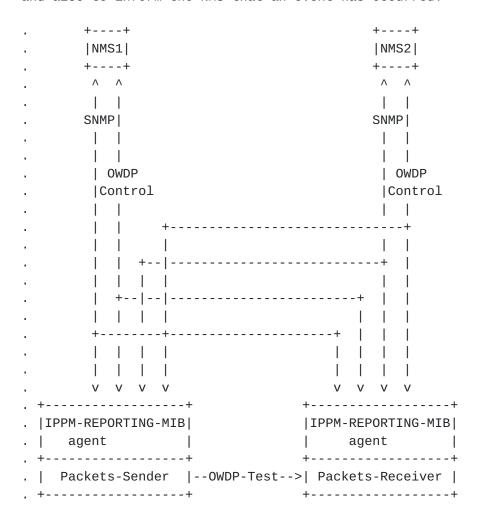
The activation of a measure by the control protocol or the test protocol creates a measure in the IPPM-REPORTING-MIB Network Measure table. The table in question may be not accessible by SNMP. In this case, a list of the measure identifiers (owner, index) is handled by the measurement software.
