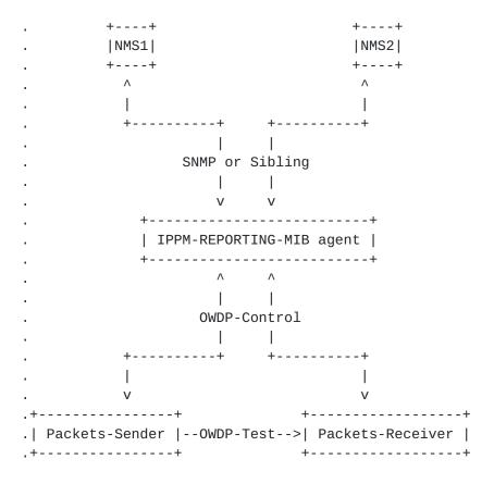
In this architecture, the different NMS s query the IPPM-REPORTING-MIB agent for measurements. The agent controls whether the NMS is granted access to perform the measure requested. Each NMS may access the results of its measurements in the IPPM-REPORTING-MIB history table.
