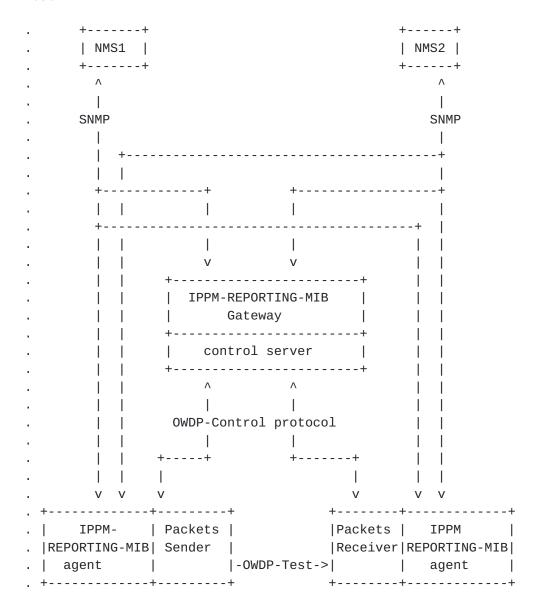
The NMS measurement queries are registered in the IPPM-REPORTING-MIB gateway and performed by the control and the test protocol. The NMS directly consults the result in the corresponding IPPM REPORTING MIB agent of the points of measure.
