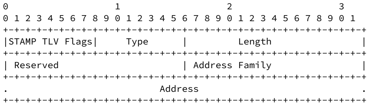
Figure 4: Return Address Sub-TLV in Return Path TLV
