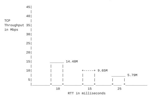
The following diagram shows the achievable TCP throughput on a 25ms T3 when the TCP Window size is increased and with the <u>RFC1323</u> TCP Window scaling option.
