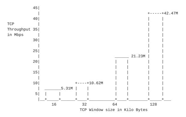
The single connection TCP throughput test must be run over a a long duration and results must be logged at the desired interval. The test must record RTT and TCP retransmissions at each interval.
