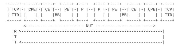
Note that the NUT may consist of a variety of devices including but not limited to, load balancers, proxy servers or WAN acceleration devices. The detailed topology of the NUT should be well understood when conducting the TCP throughput tests, although this methodology makes no attempt to characterize specific network architectures.
