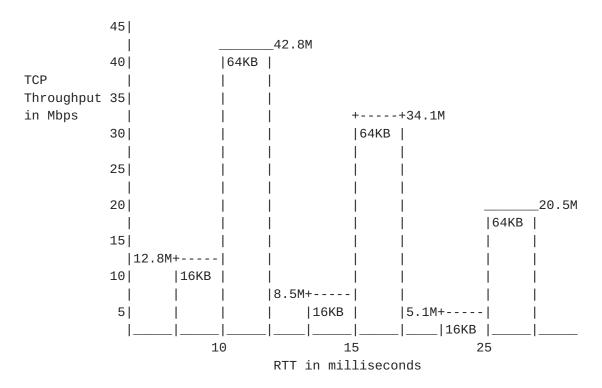
The following diagram shows the achievable TCP throughput on a 25ms T3 when Send Socket Buffer & TCP Receive Window sizes are increased.
