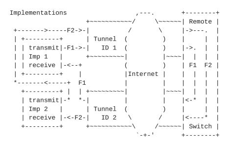
Illustrations of a test setup with a bi-directional tunnel. The upper diagram emphasizes the VLAN connectivity and geographical location. The lower diagram shows example flows traveling between two measurement implementations (for simplicity, only two flows are shown).
