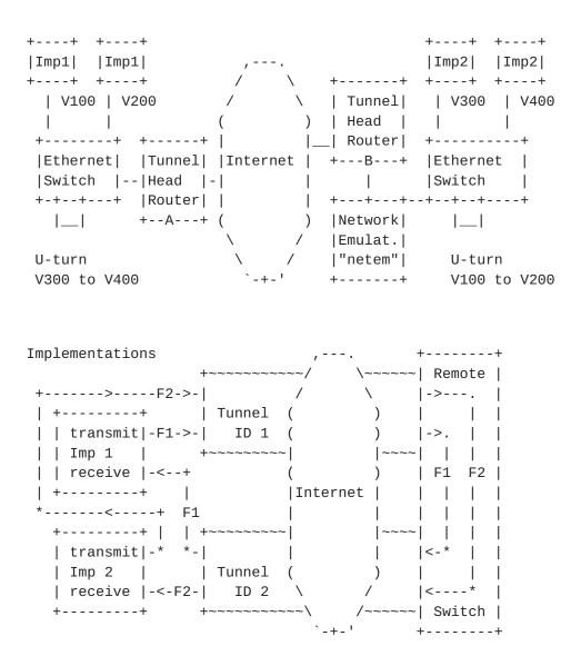
Illustrations of a test setup with a bi-directional tunnel. The upper diagram emphasizes the VLAN connectivity and geographical location. The lower diagram shows example flows traveling between two measurement implementations (for simplicity, only two flows are shown).
