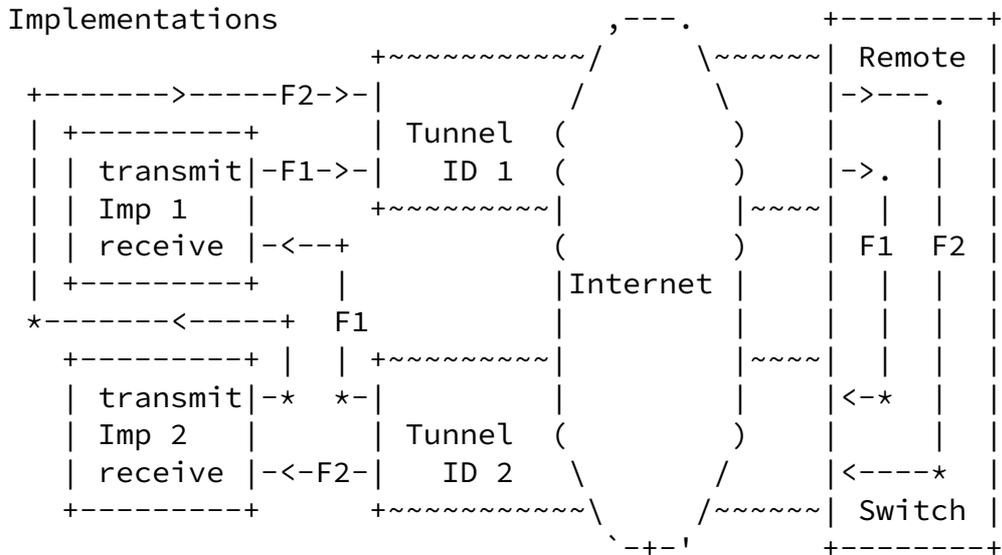
Illustrations of a test setup with a bi-directional tunnel. The upper diagram emphasizes the VLAN connectivity and geographical location (where "Imp #" is the sender and receiver of implementation 1 or 2, either Perfasp and NetProbe in this test). The lower diagram shows example flows traveling between two measurement implementations. For simplicity only two flows are shown, and netem is omitted (it would appear before or after the Internet, depending on the flow).
